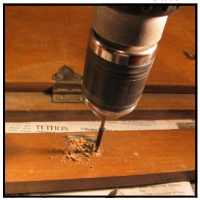
**Step 8:** Drill the pilot holes for the screws to the hinge to be mounted on the back rail of the music desk. Keep an eye on the tape to prevent the drill from going through the rail.
