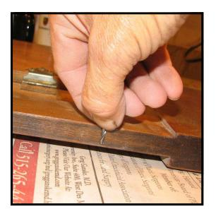
**Step 6:** For each size of screw, select a drill bit to drill the pilot holes. Placed in front of the screws, the drill should cover the body of the screw, but not the threads. Determine the depth of the holes to be drilled by actually holding the bit in front of the wood as shown. Pinch off the bit at the required point and proceed to the next step.
