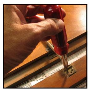
**Step 1:** Remove the old hardware. At this time, set the old hardware to one side, but do not throw it away, at least until you are sure the new replacement desk hinge is going to work properly.
