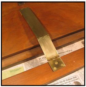
**Step 17:** With the upper segment of the hinge secured in place with screws, fold the extensions down and reinsert screws for bottom segment of the hinge.
