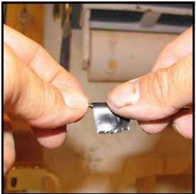
**Step 7:** Wrap electrical or masking tape around the bit at the depth chosen. Double check by holding the wrapped bit up to the wood to make sure the setting is correct.
