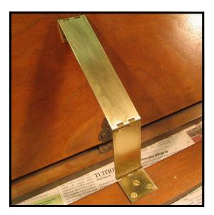
**Step 18:** Now that the hinge is secured top and bottom, pull the music rack back. The extensions should fold outward as shown in the photo.
