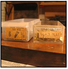
Step 5: Select the proper screws for the job. The lengths of the screws will be determined by the thickness of the rail, and the thickness of the music rack. Select screws which will not penetrate the wood, and which will fit within the beveled holes of the hinge. Brass flat head screws make the best choice for the job.
