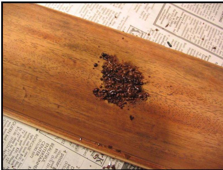
Photo 7: Melting lacquer chips start to bead up
