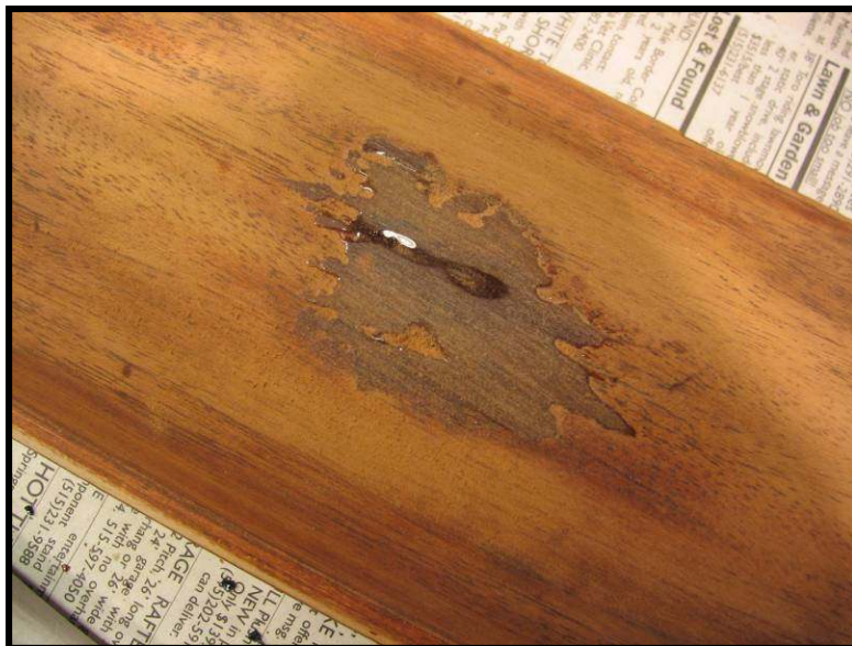
Photo 9: Sanding off the excess lacquer
