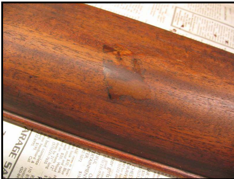
Photo 11: Staining helps blend in patch
